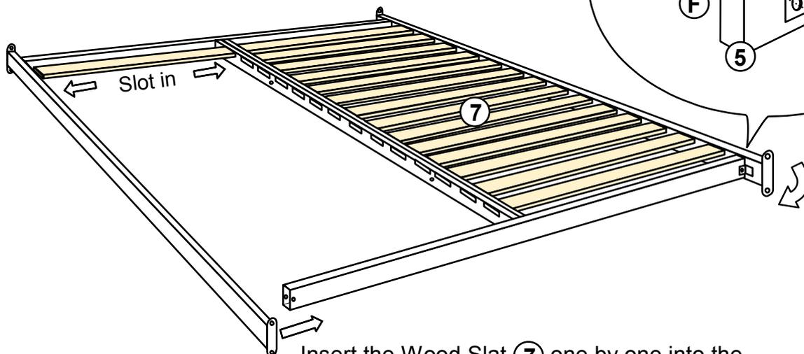
Insert the Wood Slat (7) one by one into the slots while moving the other end of the Siderail slightly inward until all 14 slats are inserted.
